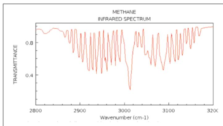
In NDIR sensors we measure the intensity of a band of wavelengths and this band is defined largely by the bandpass of the optical filters fitted to the detectors. Typically a dual detector is used which has two active elements: One is fitted with a passband filter that allows radiation which
